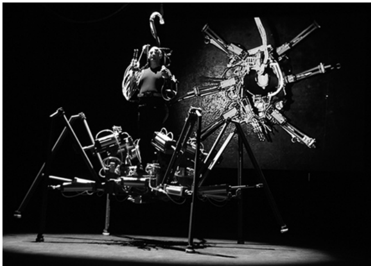
Stelarc, EXOSKELETON (Cankarjev Dom, Ljubljana 2003). The 6-legged walking machine was robust enough to support the weight of the artist. The upper body exoskeleton allows the artist to select the walking motions by his arm gestures. The robot can walk forwards & backwards with a ripple gait, sideways with a tripod gait, it can turn on the spot, sit & stand up. The performance was about taking the robot for a walk. (Photo: Igor Skafar)
