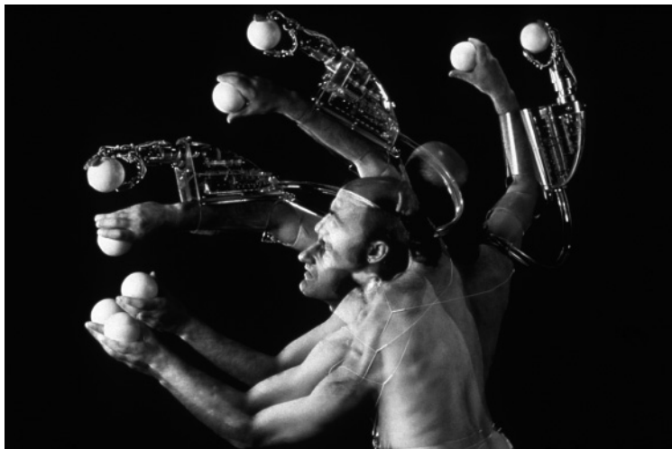
Stelarc, MULTIPLE HANDS (Roppongi Studio, Tokyo 1983). The Third Hand is a three degree-of-freedom mechanical prosthesis with a pinch-release, grasp-release & 300 degree wrist rotation, CW & CCW. Tactile sensors on the finger tips provide a rudimentary sense of touch. Originally the intention was not only to engineer a third hand but also a fourth hand to maintain the body's symmetry. (Photo: T. Ike)
