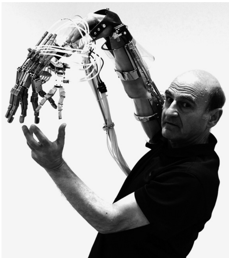
Stelarc, EXTENDED ARM (Scott Livesey Galleries 2010). The right arm is extended to primate proportions, providing the arm with an extra joint. An 11 degree-of-freedom manipulator with wrist rotation, thumb rotation, individual finger flexion with each finger splitting open, each finger becoming a gripper in-itself. (Photo: Dean Winter)
